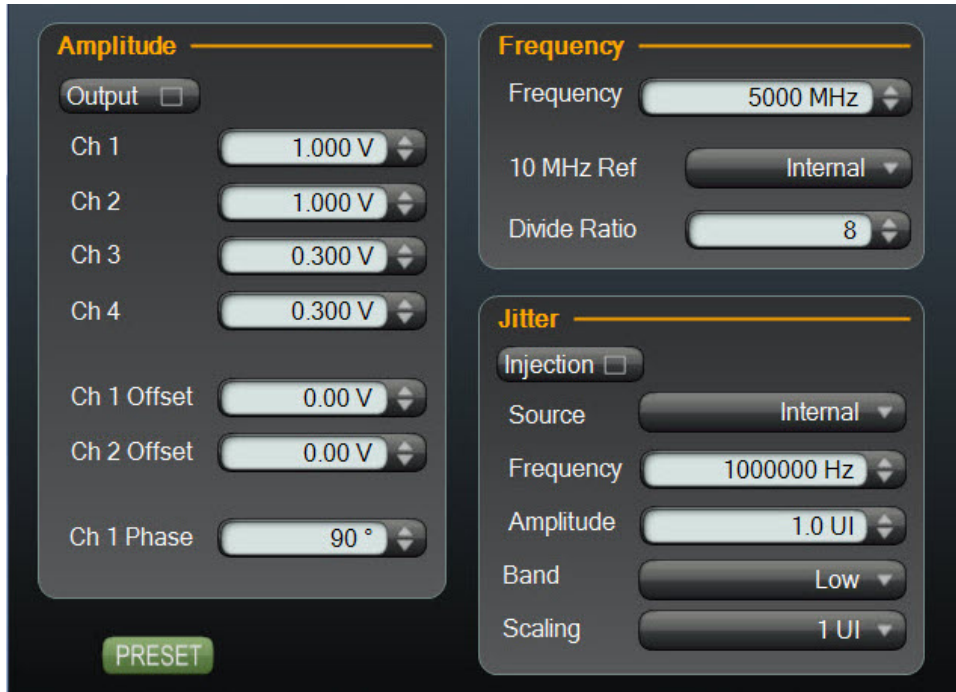
Figure 44. N4963A control panel
