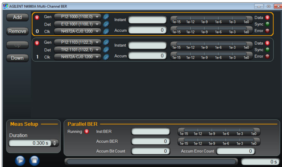
Figure 55. Multi-channel BER panel
