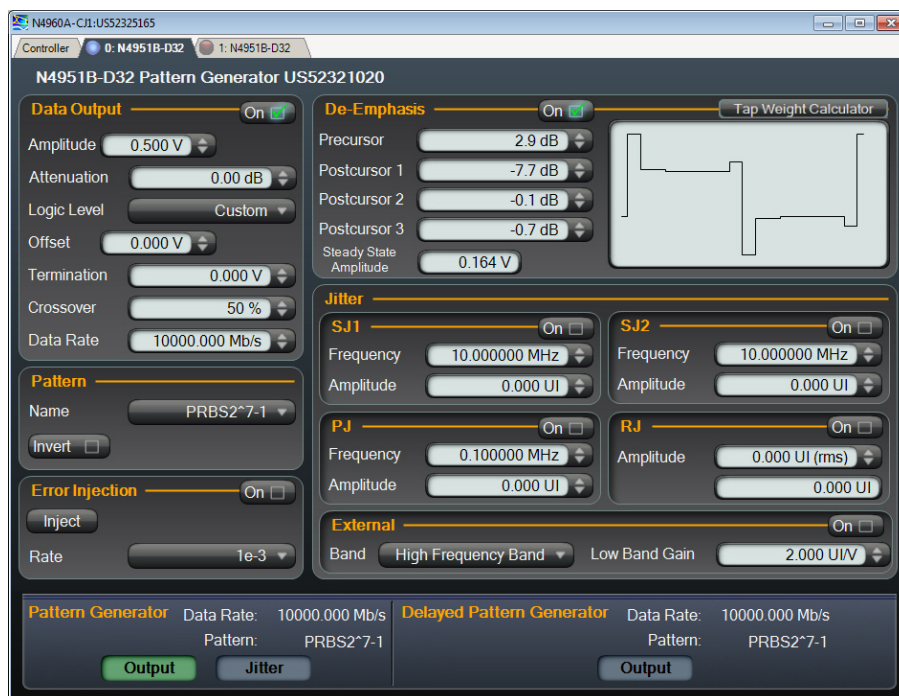
Figure 110. Access pattern generator control panel
