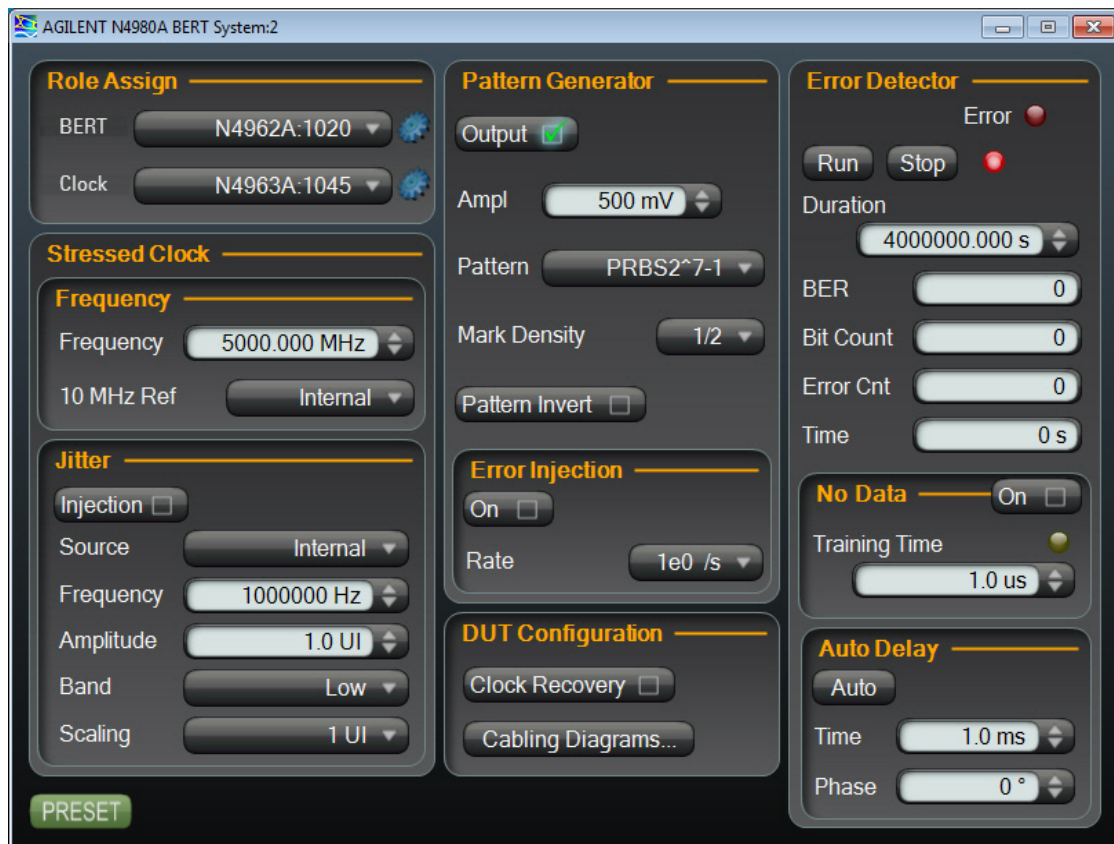
Figure 52. 10G BERT system control panel
